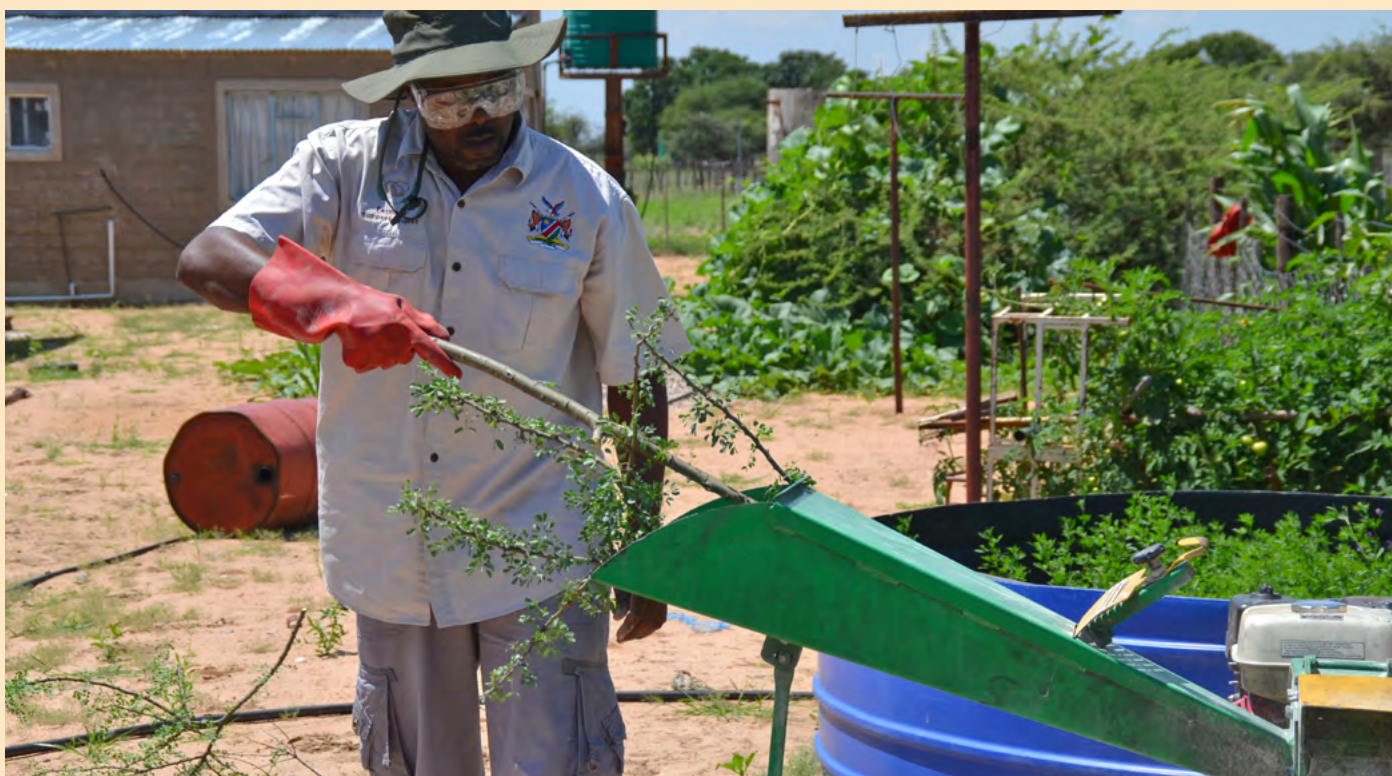
Salomo demonstrates how he uses his hammer mill machine to grind branches from encroacher species into smaller pieces for use in his animal feed.
